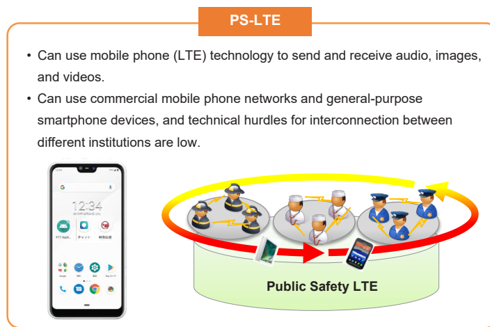
Figure 5-3-4-2 Implementation of Public Safety LTE
