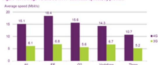
Figure 19: Average 4G and 3G HTTP download speeds, by provider
