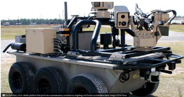
The Defender, a U.S. robotic platform that performs reconnaissance, surveillance, targeting, and threat neutralization tasks. Image: US Air Force
